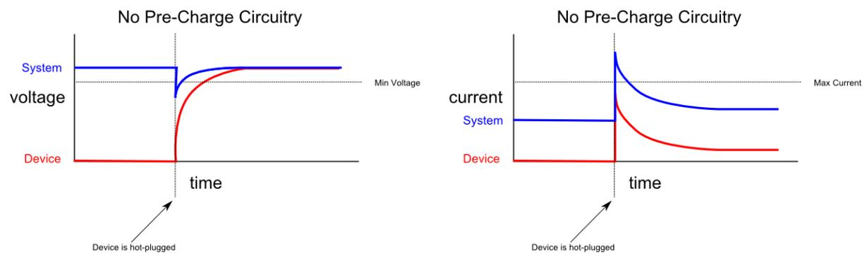
Hot-Swappable components of moderate size must employ some means of pre-charge circuitry to limit inrush current on connection. The un-charged capacitance of a 'cold' device appears as an electrical short circuit to a host system on first contact, this may cause the host system power rails to dip out of regulation or in some cases lead to complete system failure due to over-current shutdown at the power supply.
