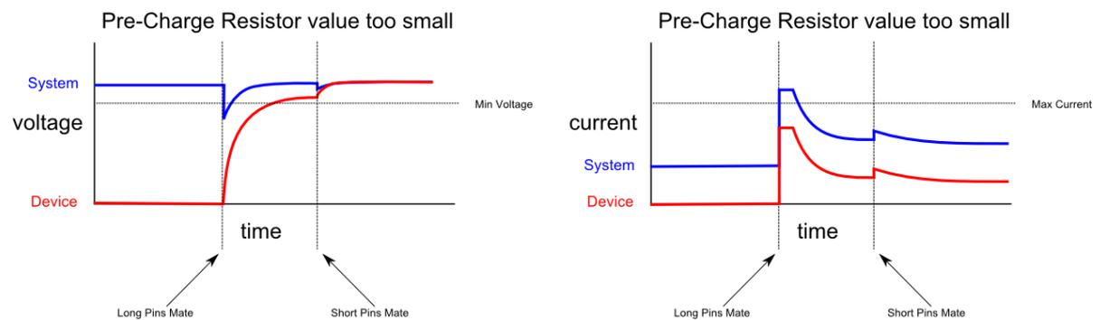
If the pre-charge resistor value is too small, the device will still draw too much current on insertion, causing the system power rails to drop out of regulation.
