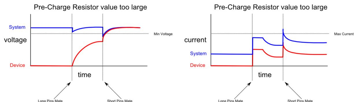
If the pre-charge resistor value is too large, the device capacitance is still not adequately charged before the power pins mate, causing the system power rails to drop out of regulation.
