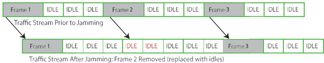
*Figure 3: Stream after Jamming to remove Frame 2 (replaced with idles)*
