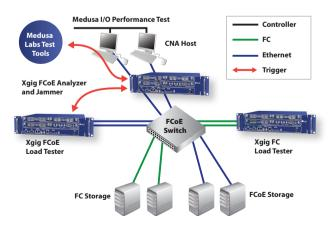
Figure 1: Example setup with the Xgig Load Tester and Medusa Lab Tools for testing FCoE switch performance.
