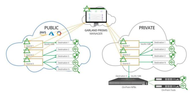
Garland Prisms virtually taps, filters and distributes cloud packet traffic to any IP address in-cloud or on-prem.
