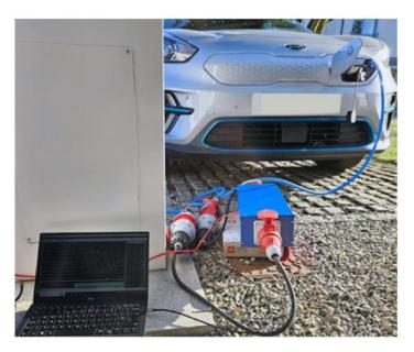
In this instance we used an EV KIA and plugged the AC PAM in series with the charging cable.
