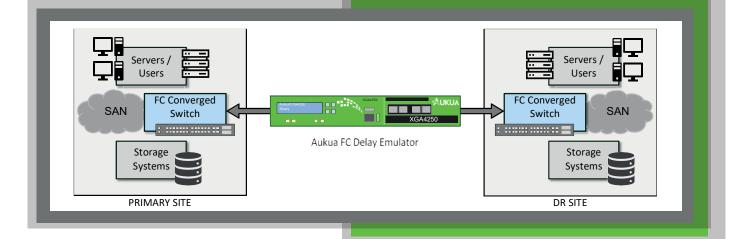
Figure 2: Fibre Channel distance emulation setup with the Aukua FC Delay Emulator
