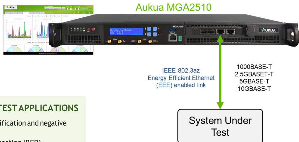
Figure 2: Aukua MGA2510 for EEE traffic generation
