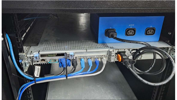
IEC PAM: SINGLE IEC 60320 C14 10A FUSED INPUT, 3 INDIVIDUALLY MEASURED IEC 60320 C13 OUTPUTS, SAMPLE RATE 8KS/S, VOLTAGE: \pm 495.5V PEAK 50VAC-270VAC \pm 0.5\% , CURRENT: 100mA-44A \pm (10mA + 0.5\%)
