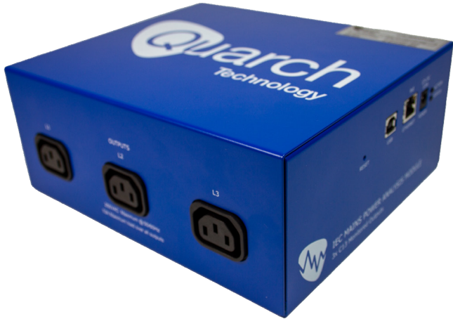
IEC PAM: SINGLE IEC 60320 C14 10A FUSED INPUT, 3 INDIVIDUALLY MEASURED IEC 60320 C13 OUTPUTS, SAMPLE RATE 8KS/S, VOLTAGE: \pm 495.5V PEAK 50VAC-270VAC \pm 0.5\% , CURRENT: 100mA-44A \pm (10mA + 0.5\%)
